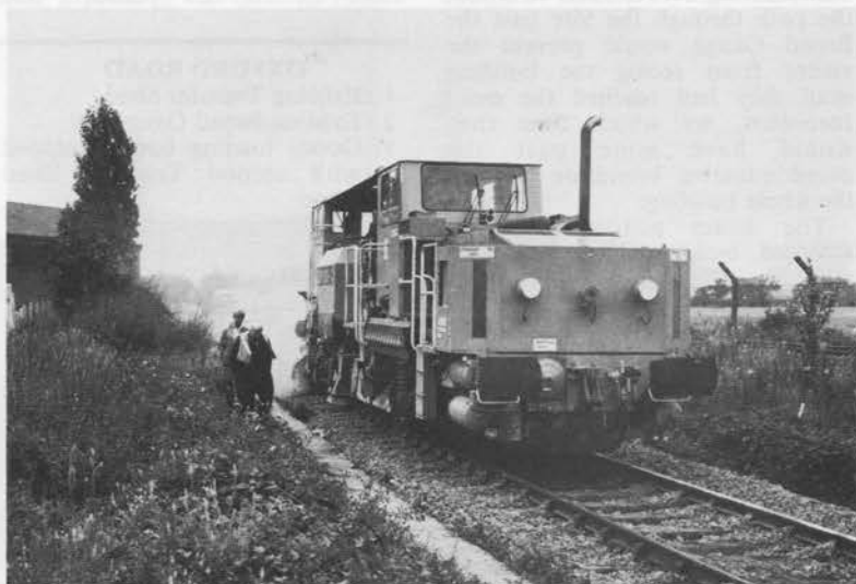
A final sweep of the Main Line extension by the BR ballast regulator in August 1986 makes for a perfect job.
